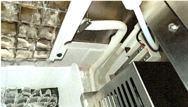
Figure 3. S2 represents the surface of the water tank at 1cm below the maximum water level.
